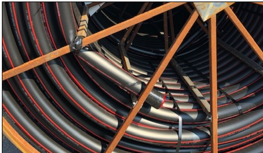
Figure 5: End of a coil of conduit showing deformation
