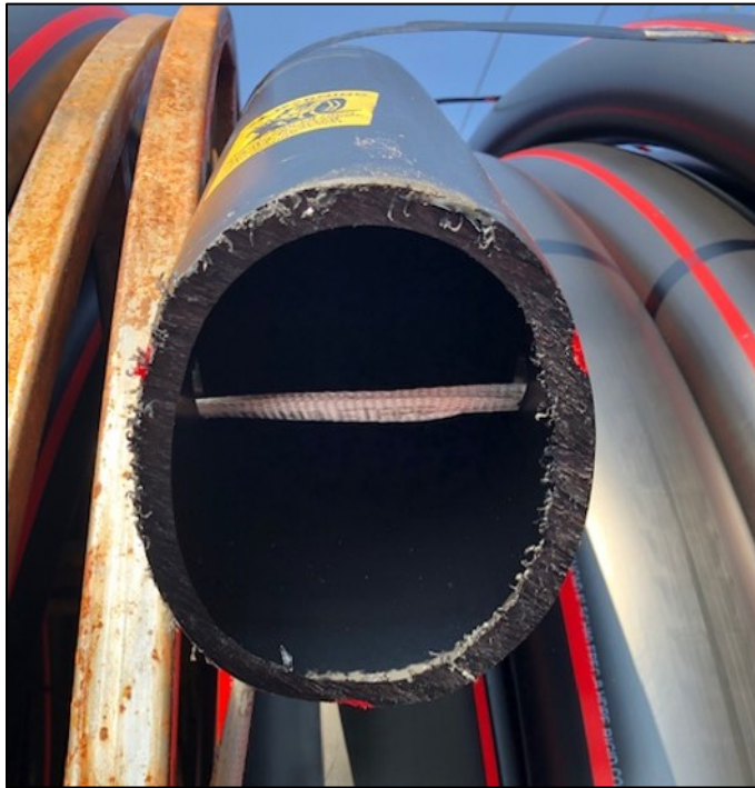
Figure 6: End of a coil of conduit showing deformation and ovality
